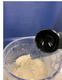
3. Add 2-5 drops Darvan to the glaze in the new container
