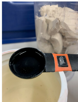
3. Add 2-5 drops Darvan to the glaze in the new container
