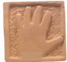
CC512R • TFJ Red (fires up to Δ8: this sample fired to Δ06)
