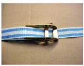
Wrap the strap around the mold. Make sure the nylon strap is not twisted! Pass the end of the nylon strap through the BACK slot at the rear of the tongue plate. There are two slots. For this step you want the one closest to the three grooves.
