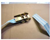
Fold the U-shaped buckle under the tongue plate. The buckle moves easily on the hinge. The crossbar of the buckle (where the nylon webbing is attached) should end up under the three grooves at the back of the tongue plate.
