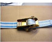
Bend the nylon strap forward again, OVER the crossbar between the two slots. Put the end of the strap DOWN through the first slot. The strap should curve into a "U" over rhe two slots.
