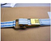
Adjust the position of the strap around the mold. You need a couple inches of slack in the strap: the next step is to flip the tongue plate forward, tightening the strap. If you don't leave enough slack for this step, it's possible for the strap to crack or crush the mold. Experiment to see what's comfortable for you, but it shouldn't take major FORCE to flip the tongue plate over and tighten the strap.
