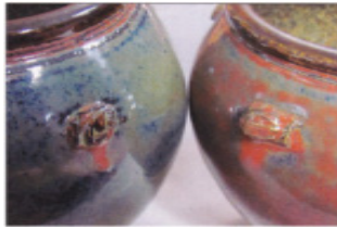
Same glaze: the left bowl had thinner application and 14 hours firing. The right bowl had thicker application and faster firing (9 hours).
