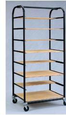
Sides are constructed from a single bent piece of heavy-walled 1" steel pipe, with welded steel shelf supports. Heavy-duty clamps connect the sides (top & bottom) with three 1" steel pipes, and 4" caster wheels. Includes a cover.
