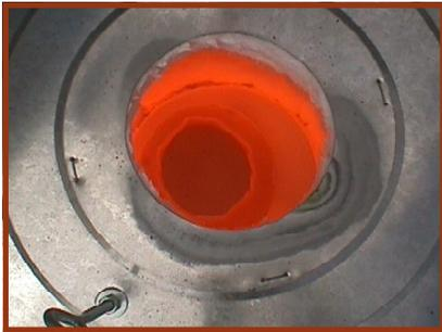
1. **PROPANE IS VERY FLAMMABLE, AND POTENTIALLY EXPLOSIVE.** Propane is heavier than air. If your fuel tank leaks, propane will settle into any lowlying areas or holes in the ground around your kiln. Be aware for any scent of propane in the area around you. We recommend that you do not smoke, and do not permit smoking, around your kiln.
